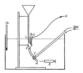
equilibrium is reached; the calibration readings are taken again with closed gas outflow tube and shaken electrode. The calibration curves are linear. In general 3 sample readings and 3 calibration curves are determined which agree closely; the time needed for one sample determination and one calibration curve is about 20 min.
